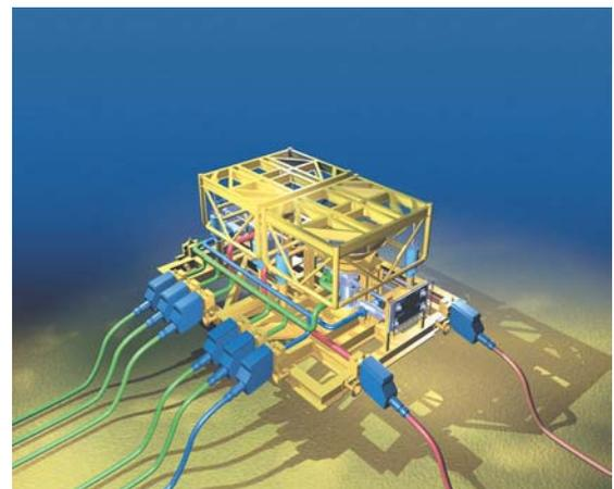
*The Flow-cap system module using conventional manifold components*
