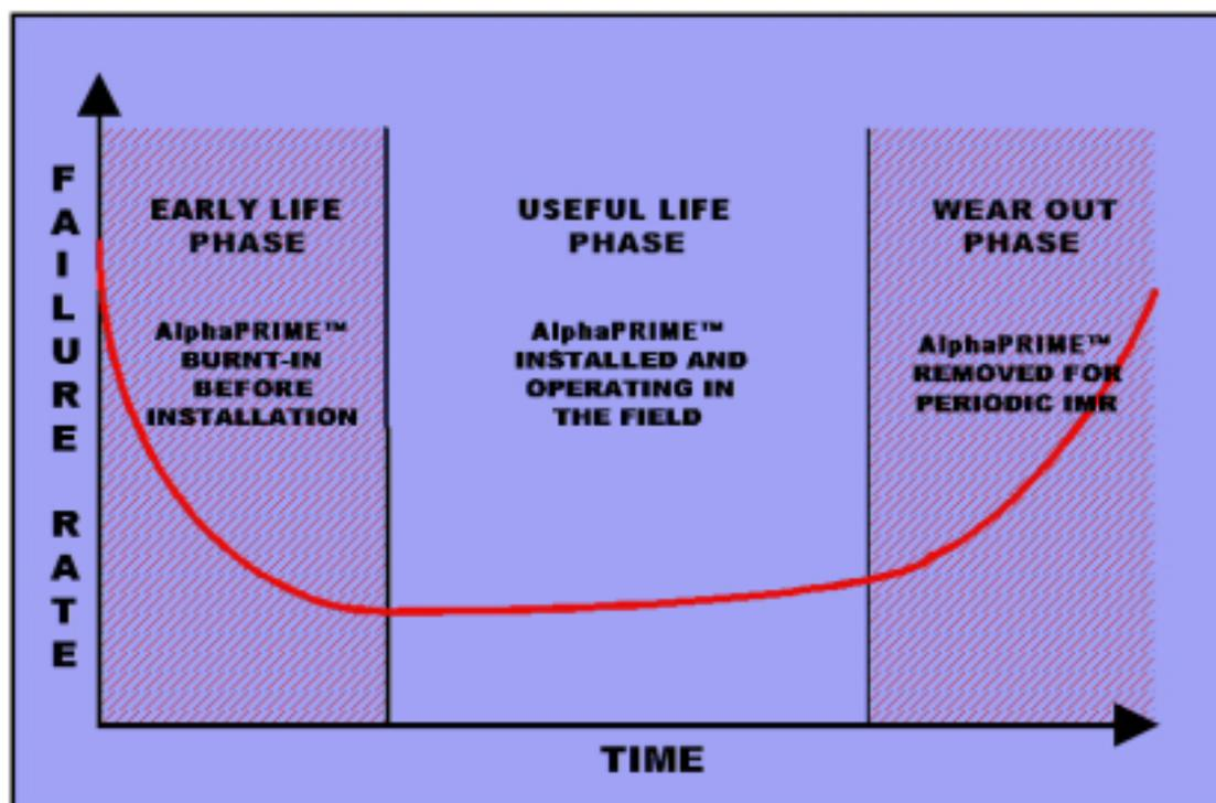
**Figure 1- Reliability “Bathtub” Curve showing the optimum reliability of AlphaPRIME™ in the field**
