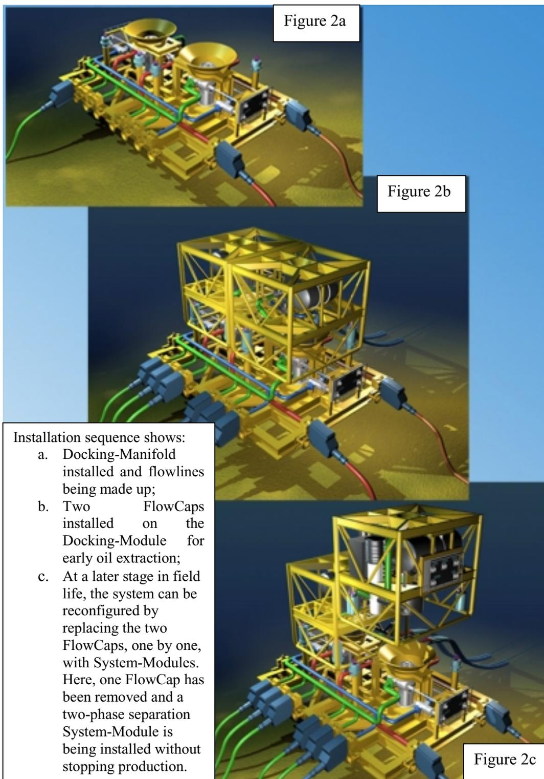
**Figure 2 – AlphaPRIME™ CPU: Installation Sequence**
